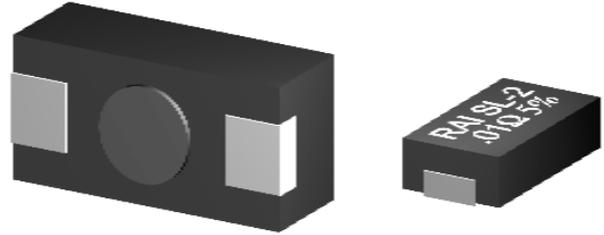
Riedon's SL and S power resistors serve today's expanding usage of surface mounted circuitry. The SL Series is for low resistance requirements from 0.005 to 1 ohm. This low-profile design uses a welded strip metal resistance element with very low inductance (0.5nH to 5nH) and low thermal emf. The S Series uses a welded wirewound element for higher resistance applications to 50K ohms.
