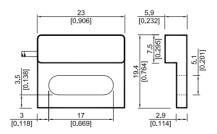
Reed Sensors with Screw Fastening Slot
